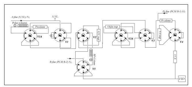
Figure 1: Reformulyzer M4 Flow Diagram
